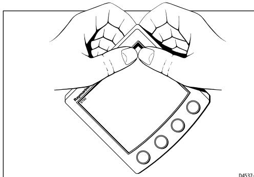
2. Using both thumbs, gently press an upper corner of the instrument from the bezel, then remove the bezel from the instrument. Retain the rubber keypad which is released when the bezel is removed.
