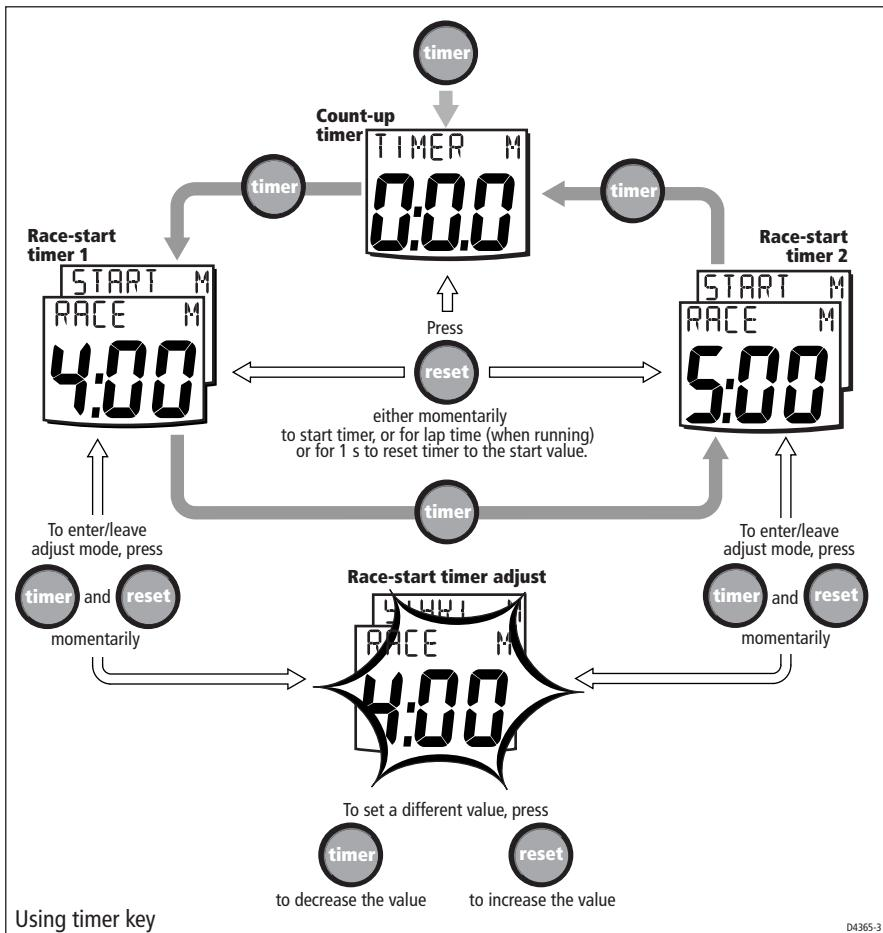
Once you have selected the required timer display, press the **reset** key to start the timer running. When a timer is running, the delimiter (i.e. '.' or ':') flashes. For lap timing, press the **reset** key. To stop and reset a timer to the start value, hold down the **reset** key for 1 second.
