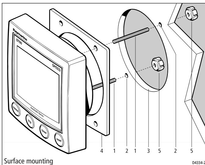
2. Apply the surface mount template (supplied at the rear of this handbook) to the selected location and mark the centers for the fixing studs (1) and the aperture (3) that will take the rear casing of the instrument.
