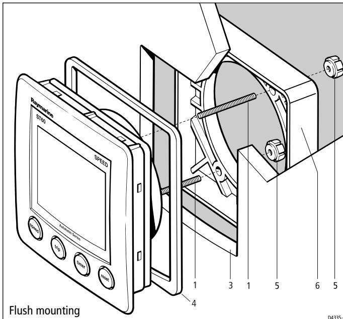
6. Screw the two fixing studs (1) into the threaded sockets on the rear of the instrument.
